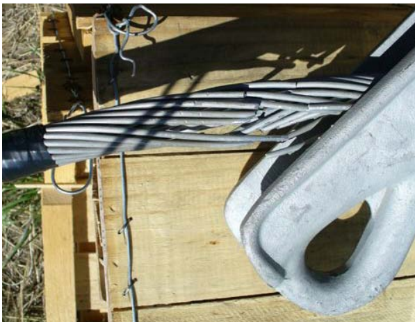
Broken and severely worn strands inside bolted, quadrant style deadends
