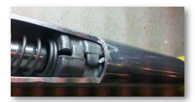
The critical concern is that <u>neither of these situations are visible or otherwise readily detectable</u>, and while the splice may hold the line under the stringing tension of a few hundred pounds, additional tension or other disturbance during work on the line may be enough to allow it to slip.
