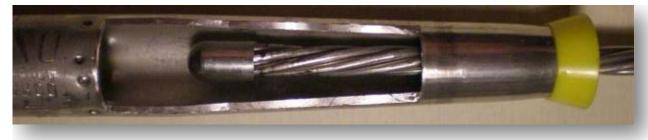
Prior to insertion, having this side cut out from the splice, one can see the position of the jaws, urged forward by the force of the spring, awaiting insertion of the conductor.
