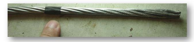
Without question, 75-80% of the problems with automatic splices occur due to installation error, and about 80% of those are "partial insertion" errors. There are two types of "partial insertion errors. The first is an <u>Incomplete Insertion</u>, where the conductor is simply not inserted to its full intended depth such that the pilot cup has not "cleared" the jaws!
