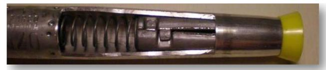
Upon insertion of the conductor, having picked up the pilot cup as it passes through the funnel guide, the "resistance" that is felt during installation is the force required to push the jaw assembly backward against the spring.
