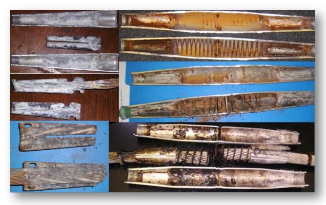
"letting go" and finding, post mortem, that they are severely corroded inside.
