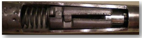
As can be seen, the pilot cup serves to maintain the conductor's position, centered within the jaws as it is pushed toward the center of the splice.
