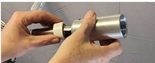
Figure 4: Plastic Spacer Install
