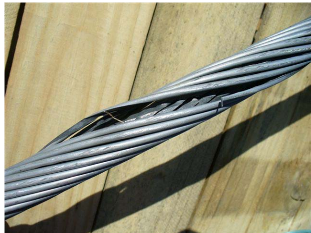
Broken and severely worn strands inside bolted, quadrant style deadends
