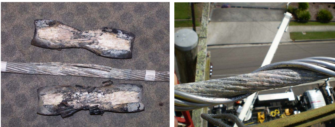
Severely corroded condition of conductor under helical rod suspension applications
