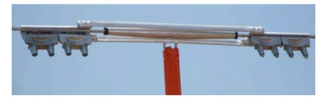
The typical side opening, inline deadend shoe, provides a clamped holding strength of 40-95% of the RBS of the conductor for which such devices are intended to be used, depending on the conductor type. The standard adopted by manufacturers has been ANSI C119.4 Class 2 Partial Tension for all bolted line hardware or strain clamps, and are tested to 40% RBS of the conductor.
